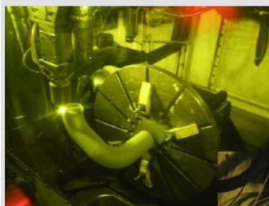
Multi Axis LMD process in continuous real-time
