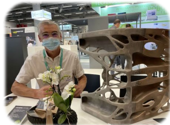
A magnesium part produced via additive casting (Ventana)
